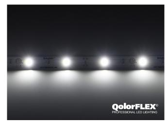
**QolorFLEX LED Tape, Cool White, 12V Indoor (P/N 5050-12-CW-30-5-20-1)** is an interior grade LED tape with a high output (515 lumens/metre) brightness. The cool white colour (6500°K) accentuates blue and subdues green and red. Each LED tape comes with wiring leads on both ends and durable 3M adhesive backing. It is available in full five metre reels and sample strips.
